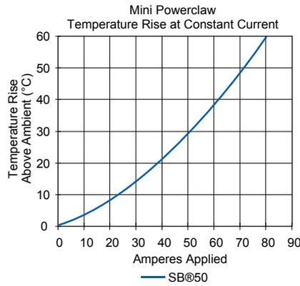
Current - Temperature Derating per IEC 60512-5-2 Test 5B
