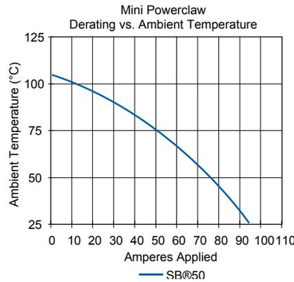
NOTE: Powerclaw charts are based on #8 AWG equivalent copper foil on board side, mated to #6 AWG conductor on wire side.
