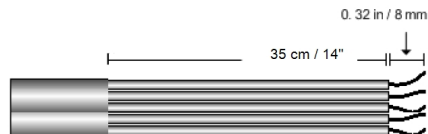
Figure 33: Insulation stripping – AC
