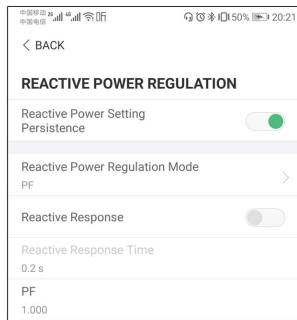
figure 7-19 Reactive Power Regulation
