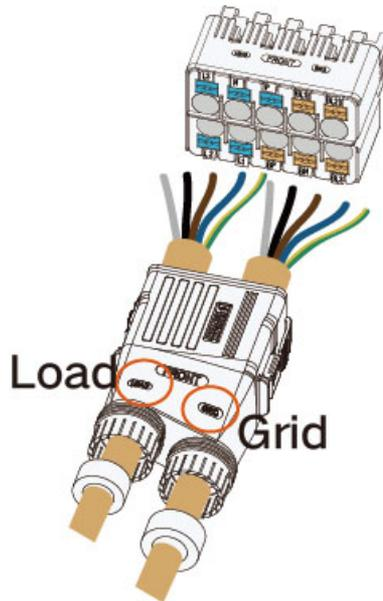
**Step 4** Strip the cable by 80 mm. If the cold-pressed terminal is to be crimped onto the cable, the cable stripping length should be 2~3 mm plus the length of the metal body of the terminal. If the cold-pressed terminal is not used, strip the cable by 14~16 mm.
