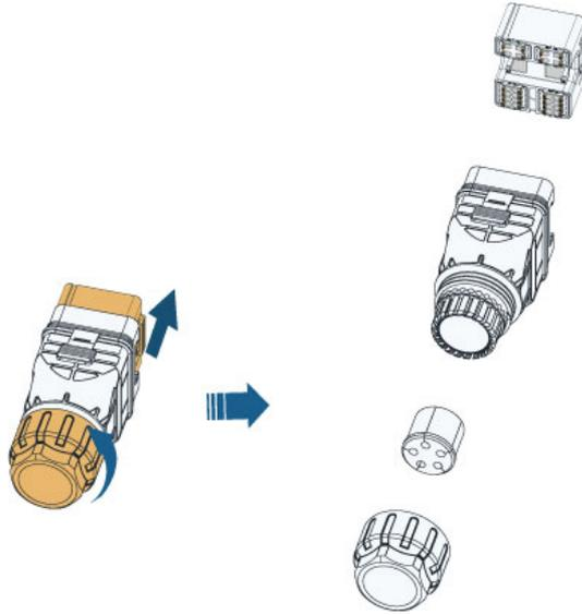
2. Remove the seal and lead the cable through the cable gland.
