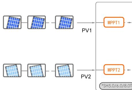
For SH10/12T, each pair of PV terminals is corresponding to an independent PV string. PV input PV1, PV2 connect to MPPT1 and PV3 connect to MPPT2. For the best use of PV power, PV1 and PV2 should be the same in PV string structure, including the type, number, tilt, and orientation of the PV modules.
