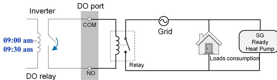
figure 8-24 DO Operation in Timing Mode Diagram
