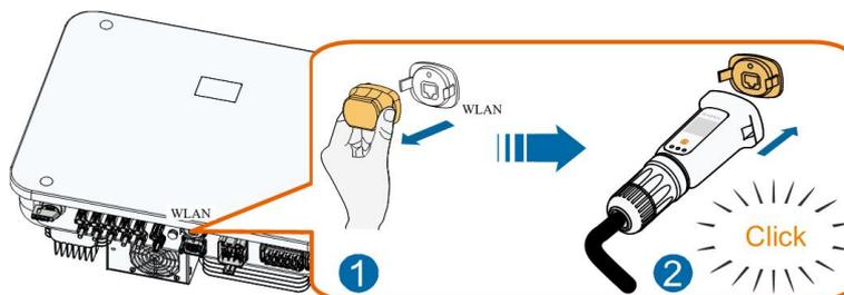
**Step 7** Slightly shake it by hand to determine whether it is installed firmly.
