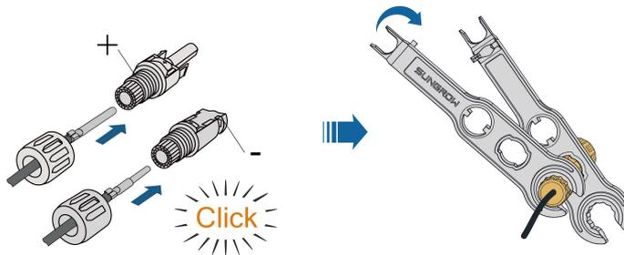
**Step 4** Check for polarity correctness.
