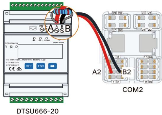
5. Insert the terminal block into the connector until it snaps into place with an audible click and fasten the swivel nut.
