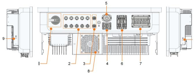
**figure 6-1** Terminals at the Bottom of the Inverter
