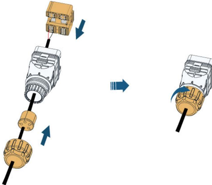
6. Remove the waterproof lid from the COM2 terminal, insert the COM2 connector into COM2 terminal of the inverter until there is an audible click.
