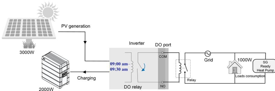
figure 8-26 DO Operation in Intelligent Mode Diagram
