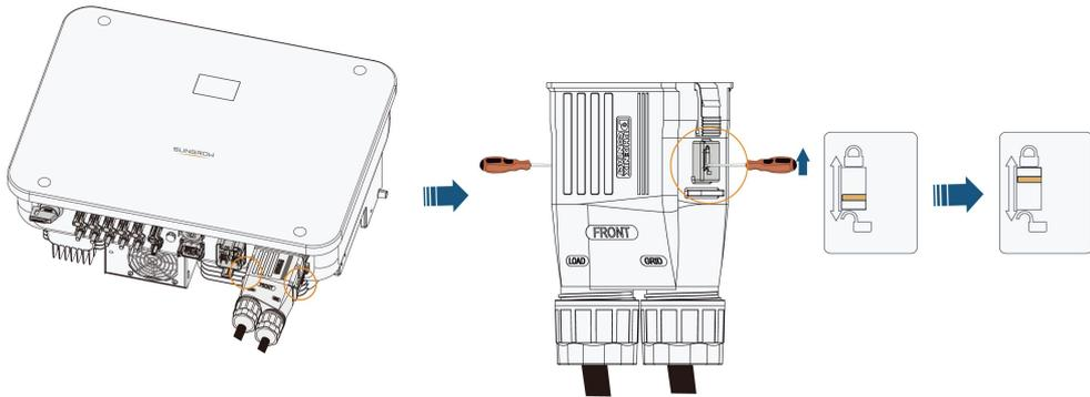
Remove the AC connector only if the AC and DC sides and the battery are powered off. Do not pull out the cable while the load is operating. To remove the AC connector, use a screwdriver to unlock it first, as shown in the figure below.
