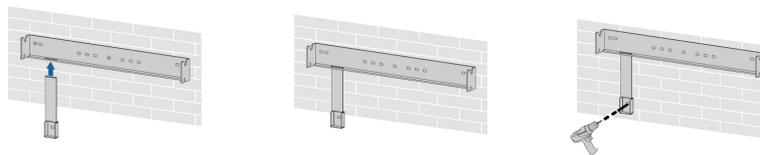
**Step 4** Lift the inverter and slide it down along the wall-mounting bracket to make sure they match perfectly. Use two screw sets to lock both left and right sides.
