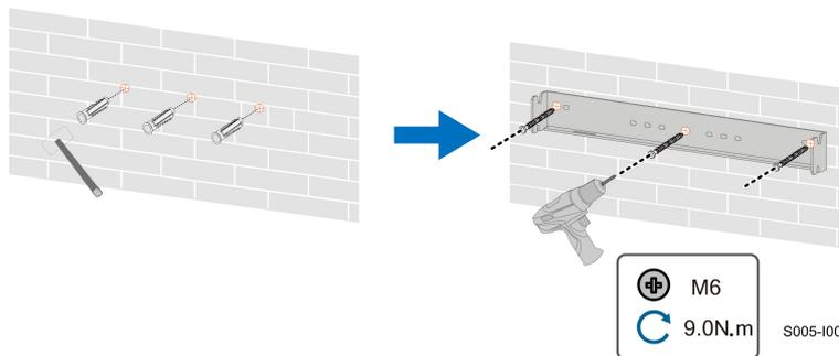
**Step 3** Install the bottom bracket to avoid the inverter tilting forward.
