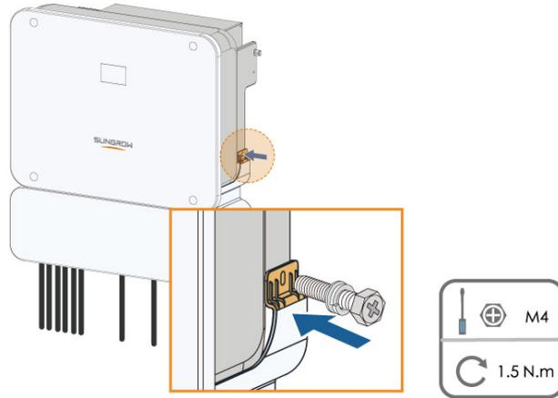
**Step 5** The installation of the protective cover is completed.
