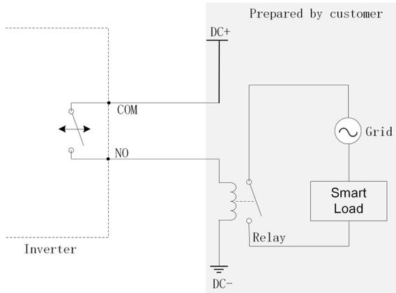
Mode 2: Use DO dry contacts to directly drive the smart load that has integrated a DI port. The maximum contact capacity of the DO dry contacts is 30 V DC@3 A.
