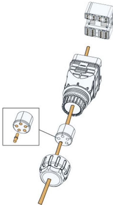
3. Remove the cable jacket and strip the wire insulation.
