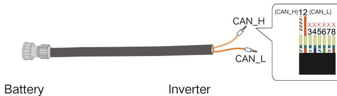
1. For usage of COM2 connector, see "[6.8.2.1 Smart Energy Meter Connection](#)". Plug the wires into the H, L terminal of the COM2 terminal.
