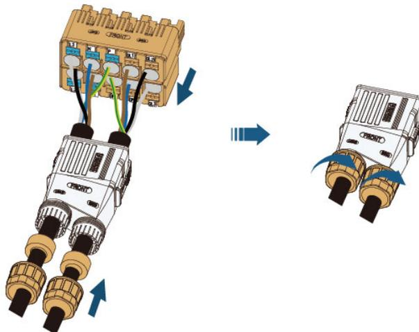
**Step 8** Insert the AC connector into the **GRID and LOAD** terminal on the inverter until there is an audible sound.
