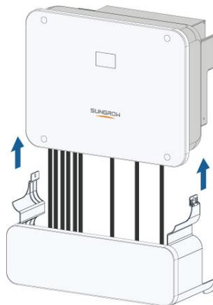
**Step 4** Use a screwdriver to secure screws with a torque of 1.5 N.m.
