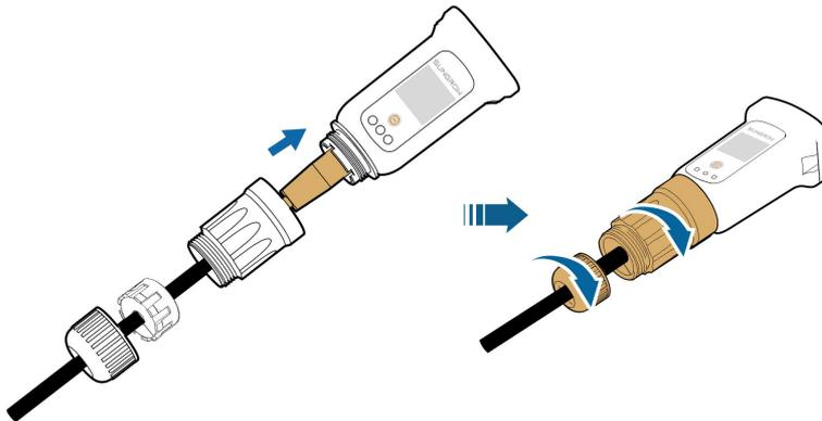
**Step 6** Remove the waterproof lid from the **WLAN** terminal and install WiNet-S2.
