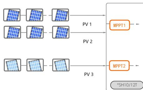
For SH15T/20/25T, each pair of PV terminals is corresponding to an independent PV string. PV input PV1, PV2 connect to MPPT1, PV3, PV4 connect to MPPT2 and PV5 connect to MPPT3. For the best use of PV power, PV1 and PV2, PV3 and PV4 should be the same in PV string structure, including the type, number, tilt, and orientation of the PV modules.
