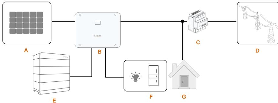
**figure 2-4** PV Energy Storage System (PV ESS)
