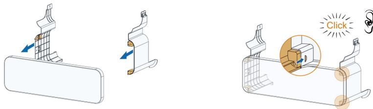
**Step 3** After the electrical connection of the inverter is completed, install the protective cover to the inverter bottom and make sure that the threaded holes in buckles of the protective cover are aligned with the holes on the sides of the inverter.
