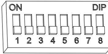
Figure 3.1. DIP Switch Block to set charging parameters
