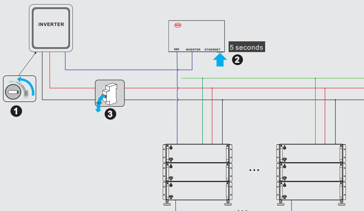
Switch Off Process: ① Inverter; ② BMU; ③ Switch between Battery and Inverter (if available)
