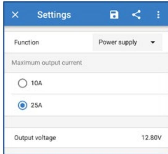
It is also possible to enable low current mode or night mode while in power supply mode and to specify the desired output voltage.
