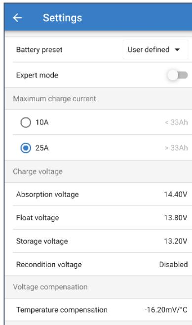
To access the advanced settings menu, open the general settings menu and enable the 'Advanced settings' switch, then select 'Advanced battery settings'.
