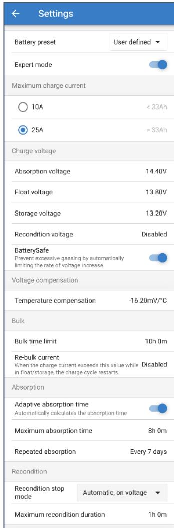
To access expert mode and expand the advanced settings menu, enter the advanced setting menu and enable the 'Expert mode' switch.
