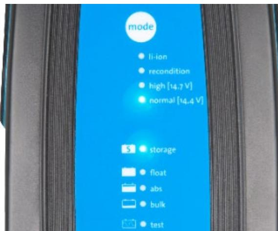
The charger will automatically store the selected charge mode and recall it for future charge cycles (even after being disconnected from power).
